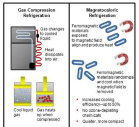
Not only will magnetic refrigeration increase energy efficiency, but no ozone depleting chemicals will be required, and eliminating the condenser will result in a quieter, more compact unit.
