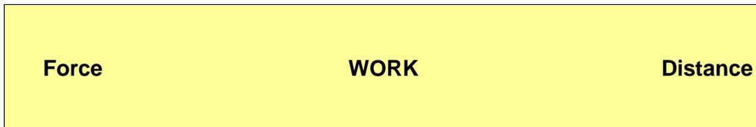
Cut out the figure above. If you hold it in the middle, it shows you that, if the force increases (raise the side with ‘Force’ on it), the distance needed to do the same amount of work decreases (the side with ‘Work’ on it goes down). If the force decreases, the distance increases.
